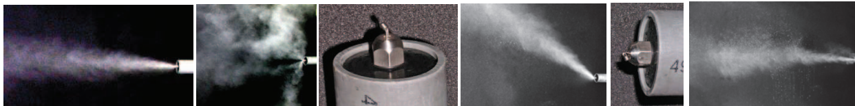
6 - Missing resonator. 7 - Plugged liquid port.
